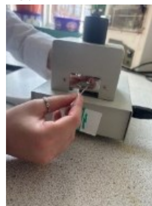
Testing purity using a melting point machine
